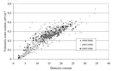
Fig. 4. Dielectric constant and the water content of the soil for the periods 1995/1996, 1997/1998 and 1999/2000
