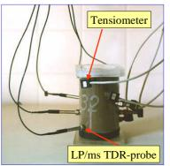
Fig. 1. Equipment for simultaneous measurement of soil water potential and soil of moisture
