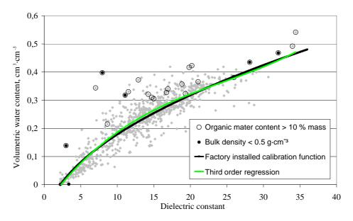
Fig. 3. Measurements compared with the factory installed calibration function concerning the dielectric constant and the water content of the
