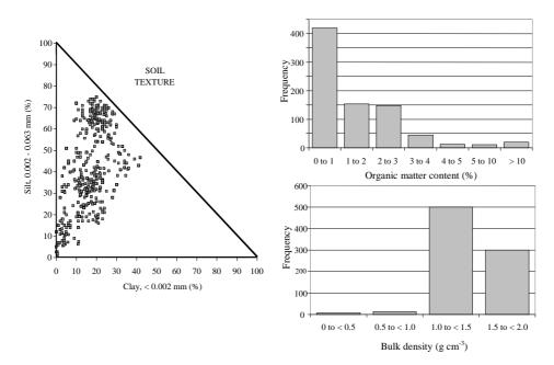
Fig. 2. Texture, organic matter content and bulk density of the tested soils
